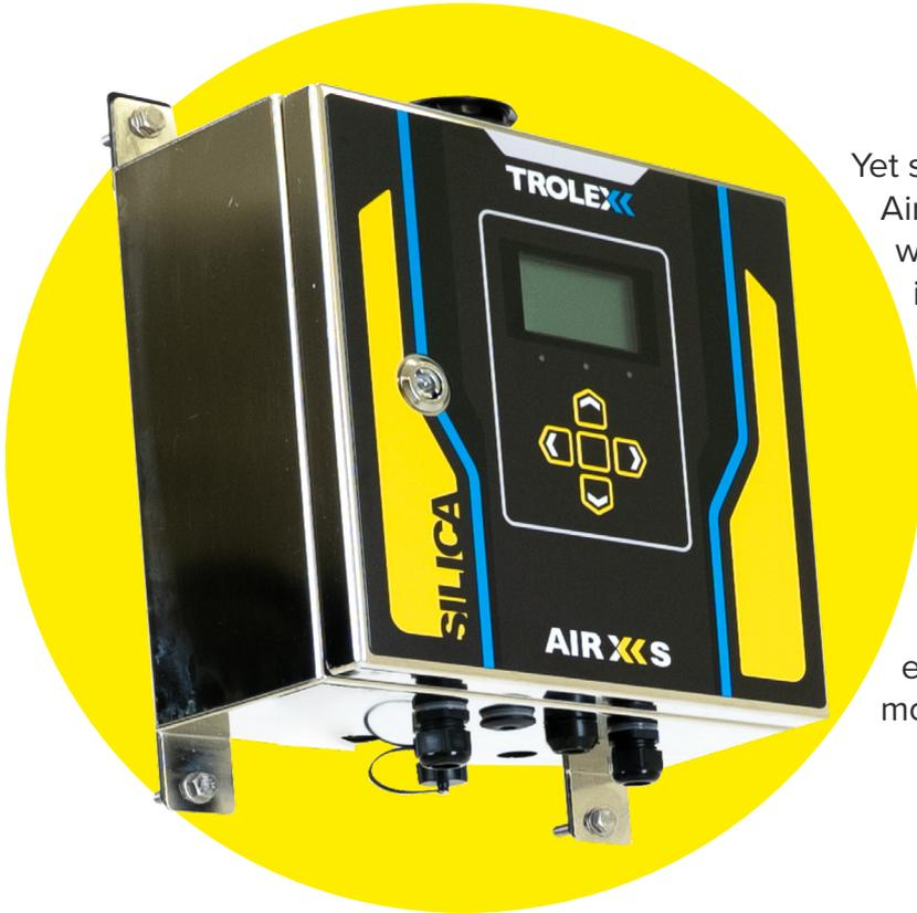
Yet silicosis\* is entirely preventable, and the Air XS Silica Monitor is set to revolutionise worker safety within the construction industry by delivering real-time detection of dangerous respirable crystalline silica (RCS) particulates in airborne dust mixtures – on the job.
